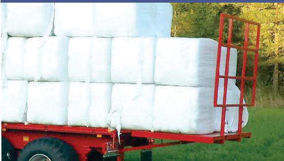
After dismantling the sides, the semi-trailer is converted into a platform that has the option of mounting bales/ pallet extensions.
