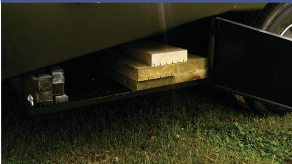
Platforms are fitted with metal toolboxes for extension sides, posts and fixing chains.
