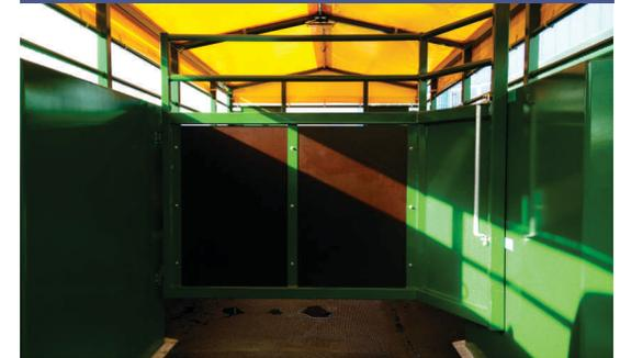
With a large amount of livestock, an internal partition with an automatic lock is closed. The partition protects animals from high movement during transport.
