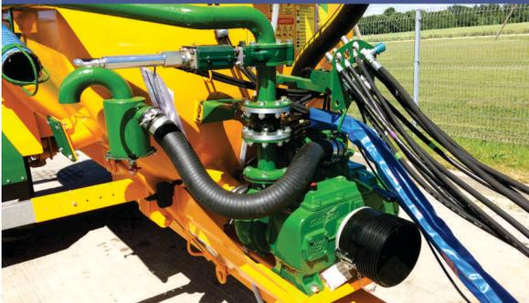
The tank is filled with a vacuum pump. The standard uses vacuum pumps from 6500 L/min to 13500 L/min performance.
