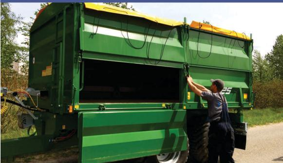
Double sides for light, bulk cargoes, single-sided sides for heavier goods, and complete removal of sides - transportation platform
