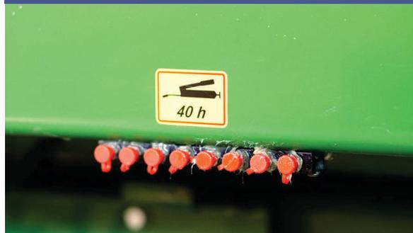
Additional add-ons – central lubrication system. All points are greased from one place.
