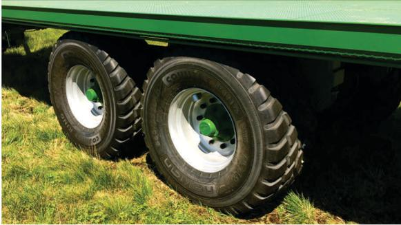
Wide and high profile tyres allow you to assemble bales in especially wet or peaty soils.
