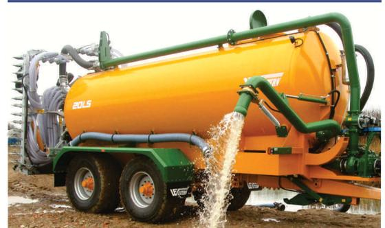
Dual pumps (centrifugal + vacuum) Used for quick filling and mixing within the container or for accurate dosing of liquid.
