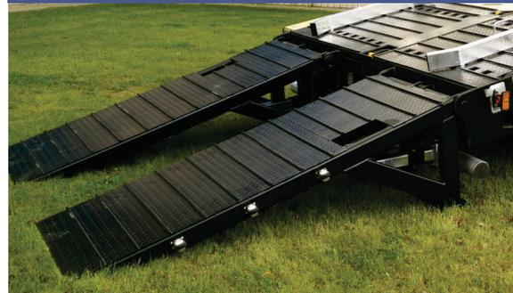
The hydraulic ramp opens directly from the tractor and forms a very small loading angle. In the transport position, the ramps are locked with an additional mechanical lock.
