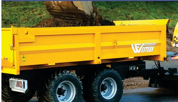
Profiled sides ensure rigidity and strength of the body when loading bulk and heavy loads.
