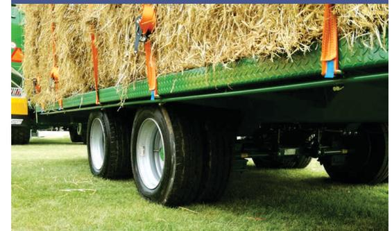
Throughout the length of the platform, the welded rods on both sides are secured to the strap fixings.
