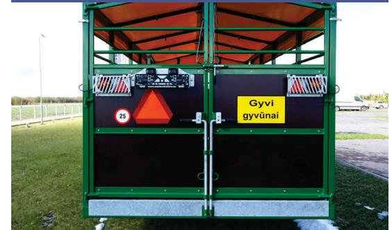
Rear doors with two powerful mechanical and one automatic lock ensure safe transport of cattle.
