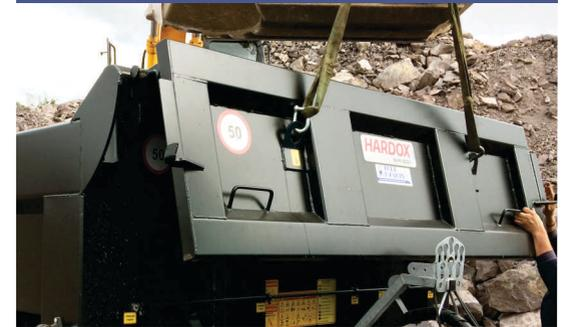
The tailboard is easily mounted on the front sheet with brackets and locked with a mechanical lock.
