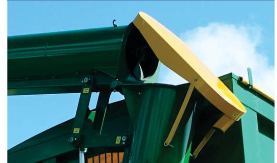
Move the auger into the transport position and cover the upper part of the auger with an automatic lid.
