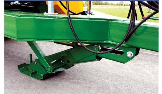
The wide-base on the hydraulic jack allows you to detach even a fully loaded semi-trailer.
