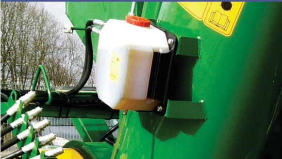
Automatic chain greasing system ensures reliable and durable chain life.
