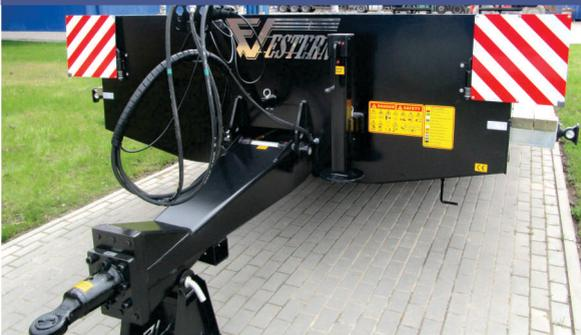
The special design of the sprung drawbar is mounted on an extremely low platform, providing greater comfort and a constant level ride on the tractor.
