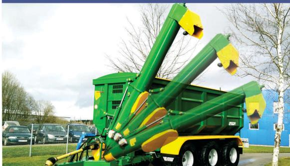
Hydraulically adjustable front discharge auger.
