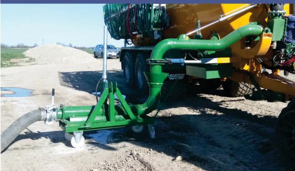
Tank-filling arm with mobile trolley is a very convenient accessory that allows you to fill the tank even without leaving the tractor.
