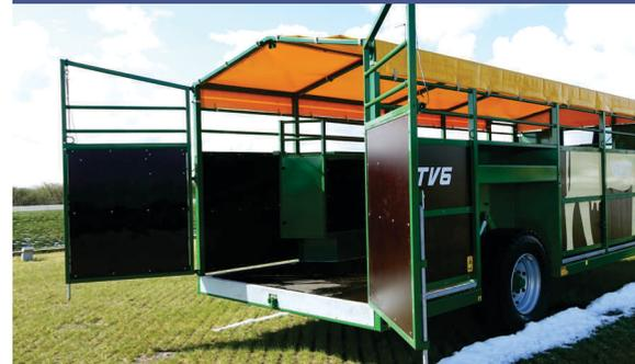
Rear doors open wide and locked into the ground.
