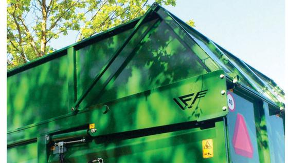
An optional accessory can be used to select the tailgate that is hydraulically opened.
