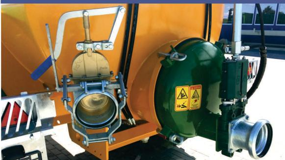
In the standard kit, the flanges are mounted on the left and right side of the tank - preparation for fill valves. The valve is available with a mechanical or hydraulic opening.
