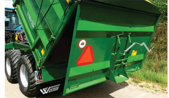
Solid rear tailboard fixed on pins at the top, the complete height of the body, with grain chute and hydraulic 300mm lock.
