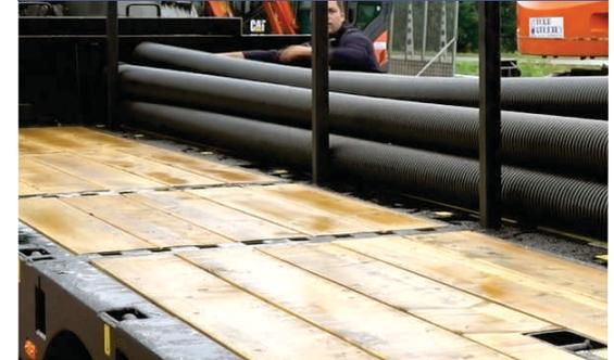
The platform has holes for posts, which are arranged so that different cargo can be transported.
