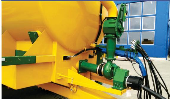
The centrifugal pump, together with the three-way valve, is used for more accurate dosing of the liquid.
