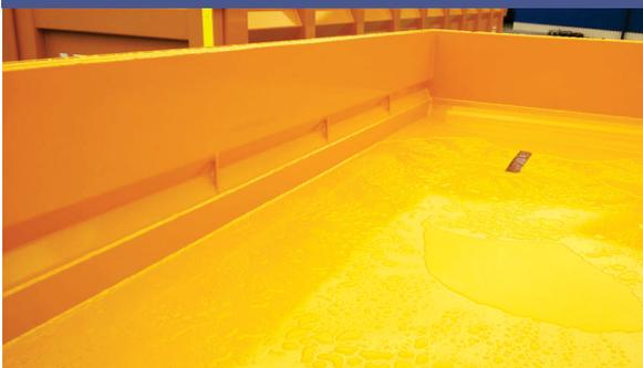
The front sheet is connected to the floor with a special bent plate – with fewer sharp corners, less load-bearing on the cargo.
