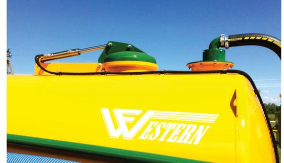
When ordering a tanker with a hatch at the top, there are two options available - a mechanically opened hatch or with a hydraulic cylinder.
