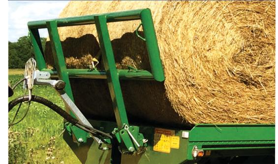
The front and rear supports are adjustable angle and are easily adapted for different loads.
