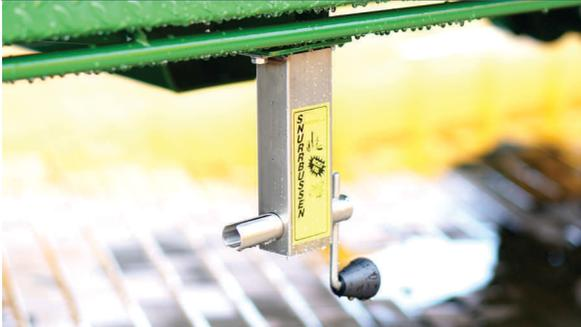
On the side of the bale-trailer is a roller belt, which will accelerate the work by wrapping the fastening belts.
