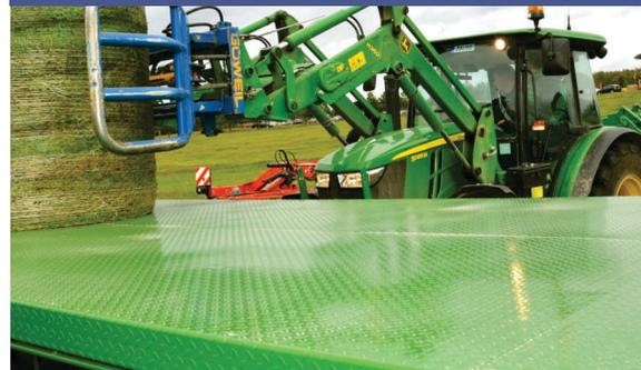
The entire bottom of the platform is made from chequer plate for increased adhesion to the loaded cargo.
