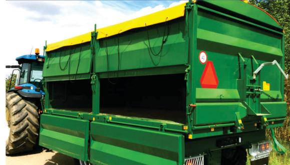
The upper side opens from the bottom, and the lower sides open upward from the bottom.
