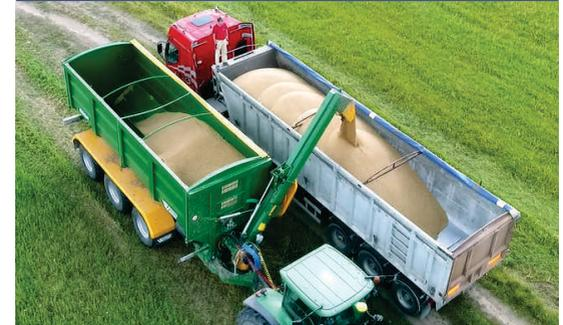
Thanks to a  $\varnothing 400\text{mm}$  diameter auger, the actual tested unloading power is 500 t/h.
