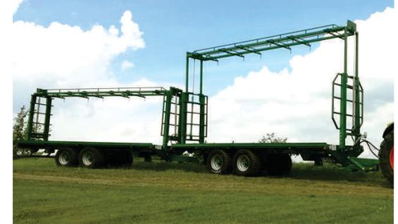
The mounting of rolls or square bundles with belts can be replaced by a quicker and safer attachment with a hydraulic press.
