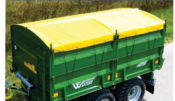
A swift and easy-to-use, tight-fitting tent is easily opened and closed from the ground. The sheet handle is conveniently attached to the body.
