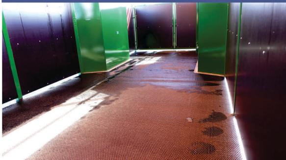
The damp-proof rubber mat and a gap between the floor and the sides facilitate the cleaning of the semi-trailer.
