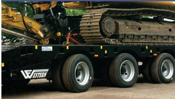
The three-axle platform can be fitted with rear and front steering axles.
