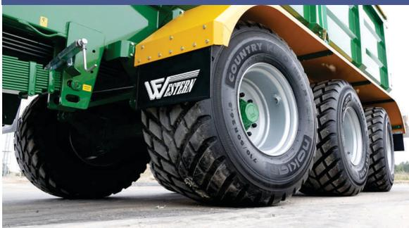
Self steering axles reduces tyre wearing and deformation when turning.
