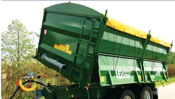
Reinforced design three way tipping with mechanically limiter for side tipping.
