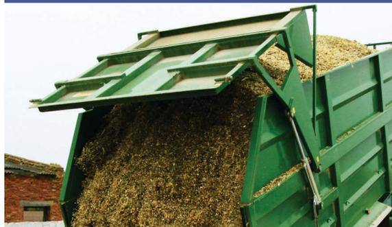
Extremely upright hydraulic tailgate with rubber seal and grain chute.
