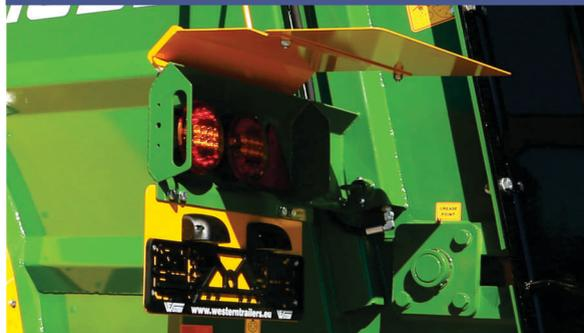
When using the hydraulic door, the cover on the rear lamps automatically closes and protects from the manure, then the lamp remains clean during transport.
