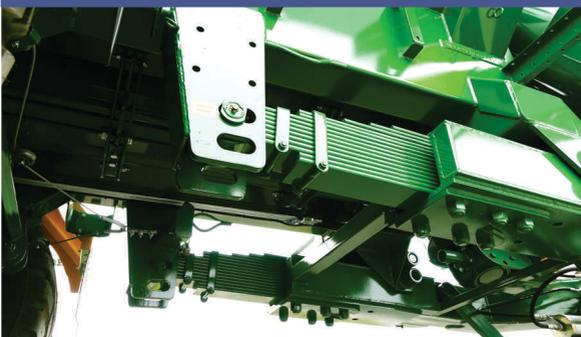
For greater comfort and smooth running of the tractor, a drawbar with two longitudinal springs.
