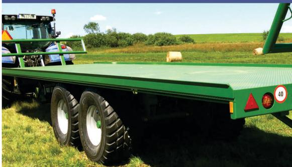
Ship plate welded on the sides of the platform protects the load from slipping during turning.
