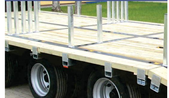
The galvanized extensions are easily removed and extends the platform up to 3 m wide.
