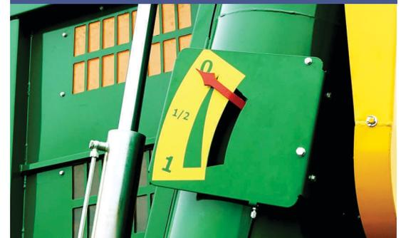
Horizontal discharge auger dispenser position indicator.
