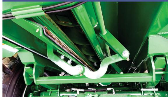
Bunker cleaning along the whole body. Opening with one handle.
