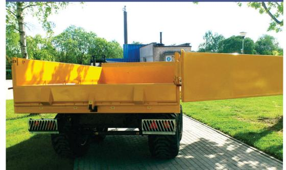
The tailboard is equipped with a mechanical or 300mm hydraulic lock, the tailboard can be opened to the side.
