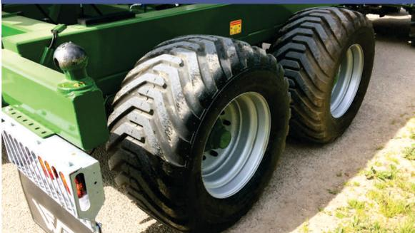
Stable sprung chassis, with the required strength axles and wide wheels.
